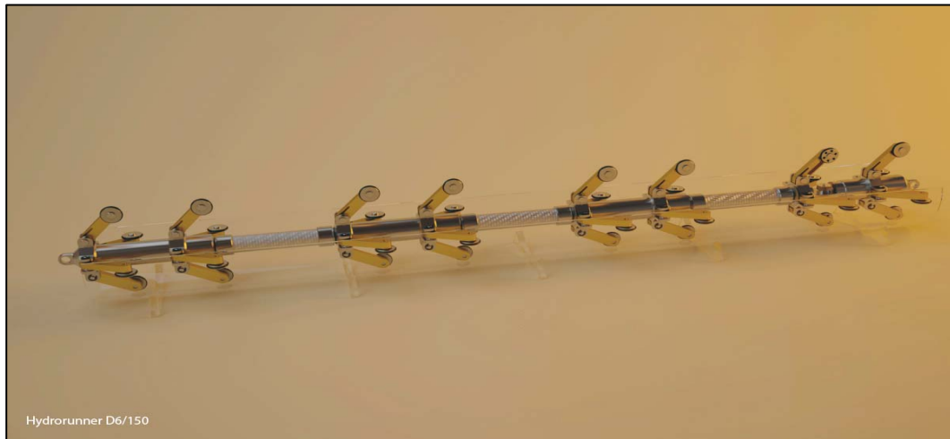
Figure 2. - A 15.24 cm (6 inch) Diameter Smart Probe Capable of Negotiating a 2 D Bend Radius.
